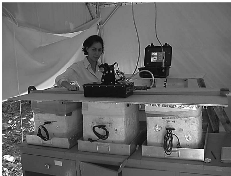
Fig. 2. Acquisition with GPR: the 900 MHz shielded antenna was passed on the soil blocks surface. The unit control from GSSI can be seen at the back.
